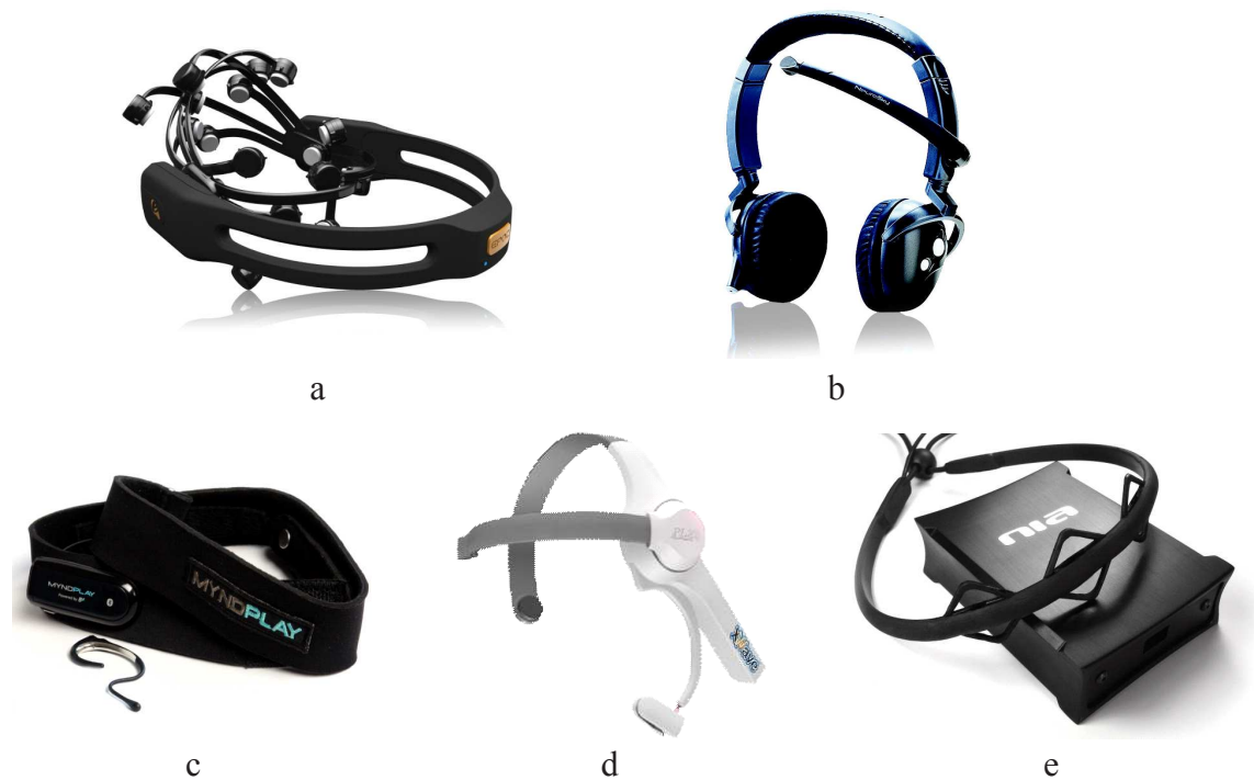
Figure 5. Pictures of Wireless BCI systems for consumer use: (a) Emotive EPOC headset [38], (b) NeuroSky Mind Set [46], (c) MyndPlay Brainband [50], (d) PLX devices XWave headset [49], (e) OCZ Neural Impulse Actuator [51].
